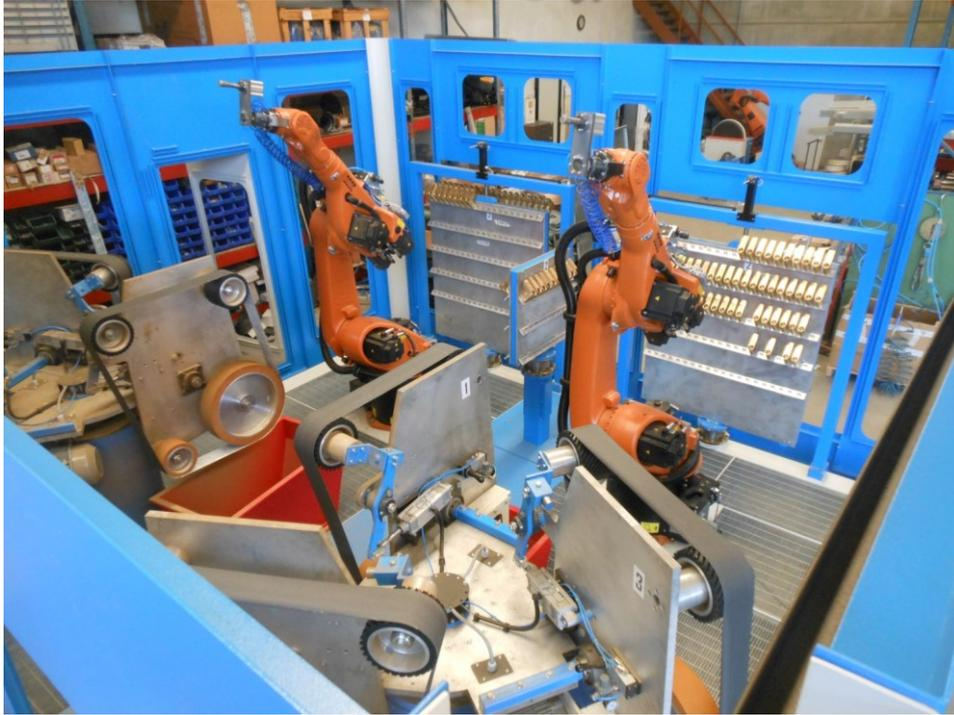
Double robot for grinding of faucets where the first robot is used to make the coarse grinding and the second one to make the fine grinding. In this way, it is possible avoiding the excessive overheating of the pieces and all the problems coming out from the high temperatures.
